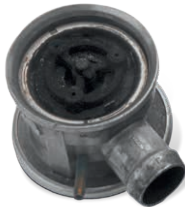
Damage as a result of exhaust gas condensate
