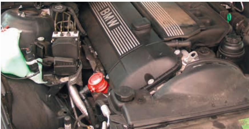
Two variants of the secondary air system
