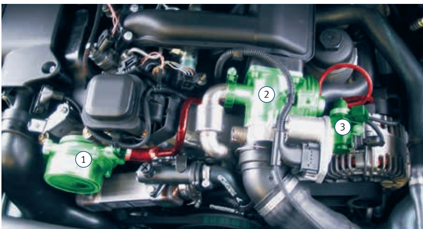
Example BMW 118d (E87): Components in the vacuum system (green), vacuum hoses (red)
